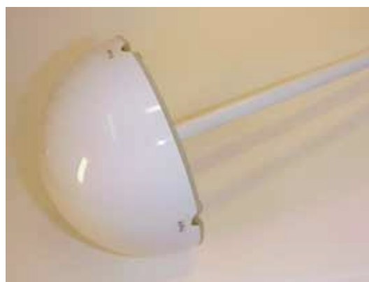
Figure 26. The phantom with the cover in place.
