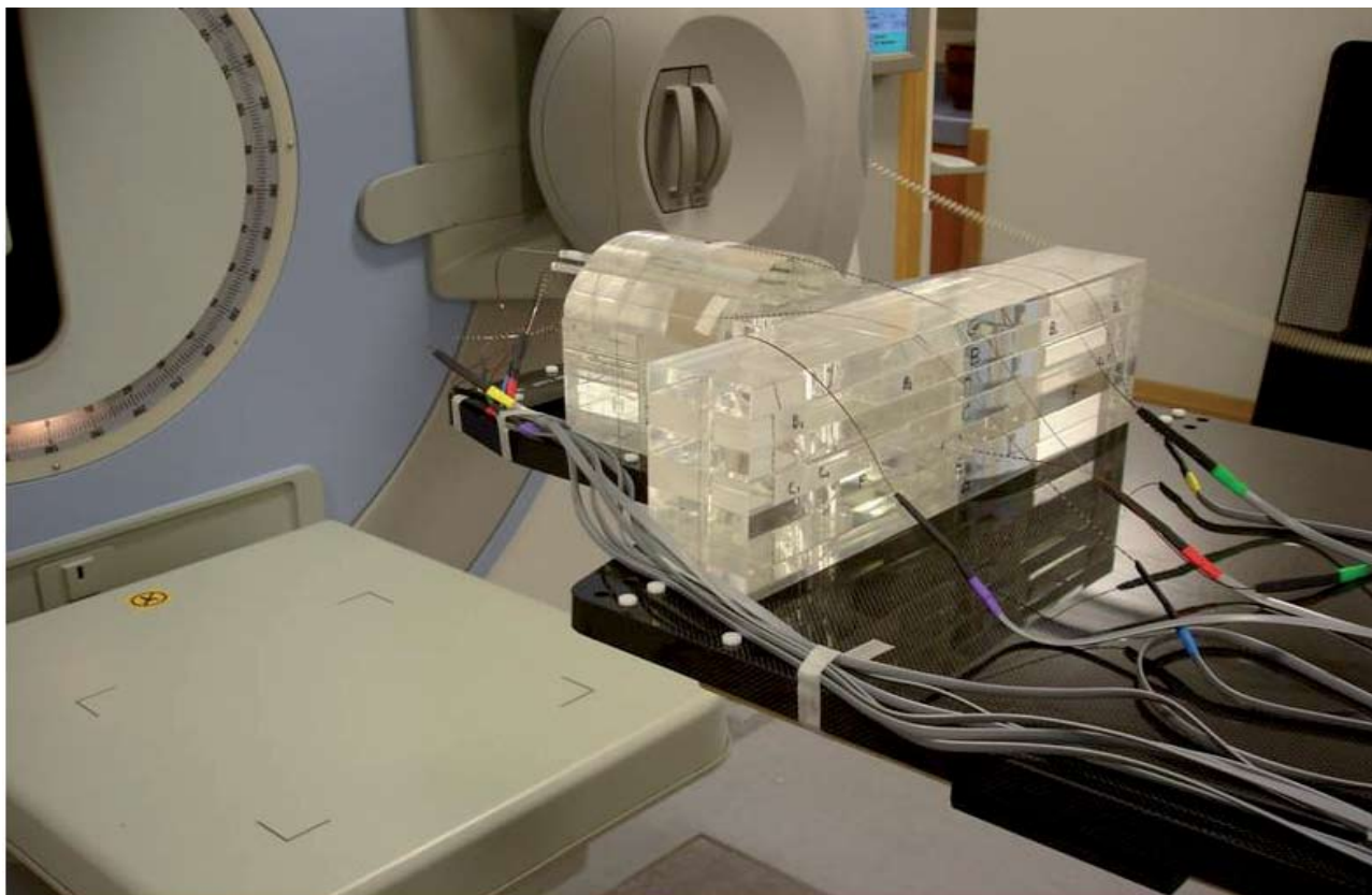
Figure 1: the perspex head-and-neck phantom (HANK) in the treatment position – the micro-mosfet lead wires can also be clearly seen.
