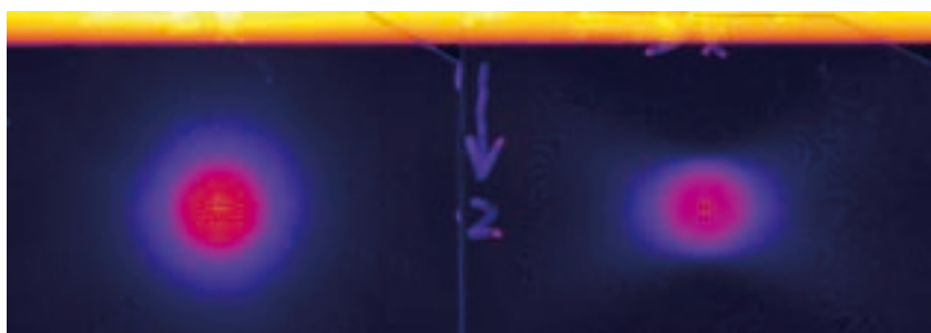
Fig 2: Radiological accuracy is determined by measuring the distance between the hole in the film and the edge of the dose distribution. According to the results presented in this report, the average value for Leksell Gamma Knife® is 0.15mm.
