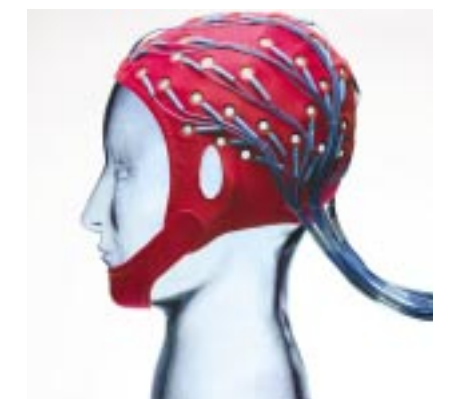
The detector array of the Eleka Neuromag® system comprises triple-sensor elements that are evenly distributed over the entire head. The size and extent of the detector array ensure that activities from even the most peripheral areas, such as frontal and temporal lobes and the cerebellum can be acquired with high precision.
